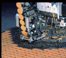
Sequin Device ☒ Embroidering various sequins: small-diameter sequins, large-diameter sequins, irregular-shaped sequins and eccentric sequins
